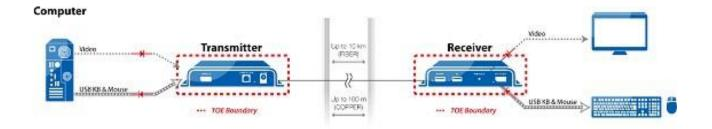
Figure 3: Isolator Evaluation Configuration
